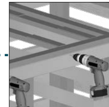
Connect with self-tapping screw (ST02)
